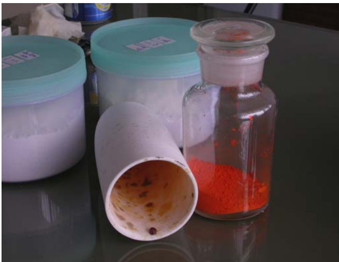
Used crucible showing yellowish to orange glass after heating.
