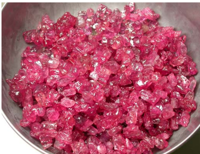
After heating, the chemicals form a glass coating as seen in this dish of ruby rough.
